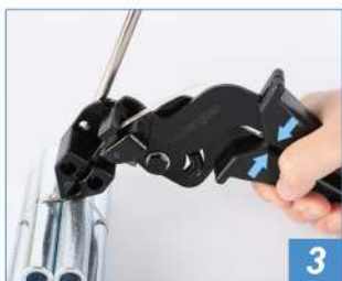
3 Insert the end of the binding band into the opening of cable tie gun hole, the gun handle in your right hand and repeat the clenching until the binding band is tightened
